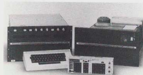
MCI/Quantel DLS 6030 digital library system with production effects. The 6030 and other units in the DLS 6000 series can now be connected to a new Central Lending Library with on-line capacity of over 100,000 still video pictures, which can be searched in under five seconds.
